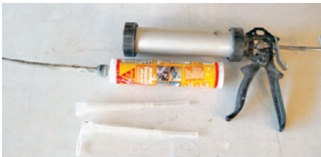
Figure 4. The author's crew used two types of epoxy — a two-part from Hilti (left) that is installed with a proprietary gun and a single-part from Sika that is delivered with a standard sausage gun (right). The long nozzle on the Hilti gun was helpful for injecting the epoxy through the thick window bucks.
