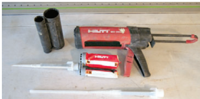
Figure 4. The author's crew used two types of epoxy — a two-part from Hilti (left) that is installed with a proprietary gun and a single-part from Sika that is delivered with a standard sausage gun (right). The long nozzle on the Hilti gun was helpful for injecting the epoxy through the thick window bucks.
